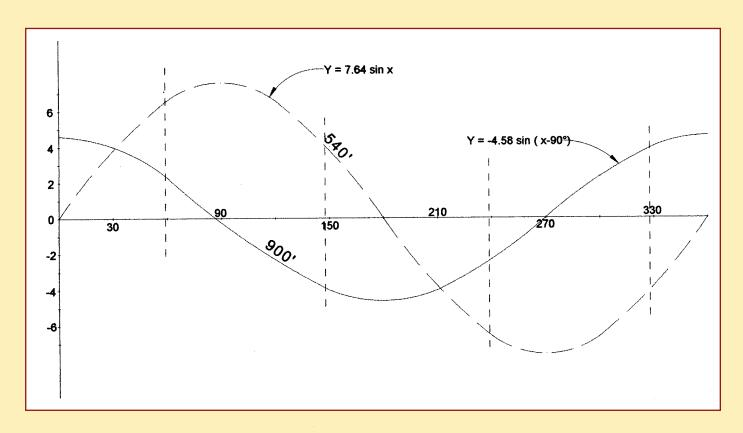
PLOT HOW EACH DIRECTION IS AFFECTED INDIVIDUALLY, AS ABOVE. (I USED 30° INCREMENTS.) THE CURVES AND EQUATIONS GIVE SECONDS OF ARC. IF THE TWO EQUATIONS ARE ADDED TOGETHER AND SET EQUAL TO ZERO, A MINIMUM VALUE WILL BE FOUND:
